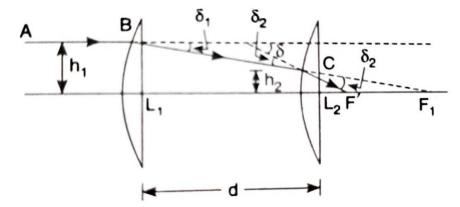
Spherical aberration can be minimized using two plano-convex lenses separated by a distance as shown in figure.
