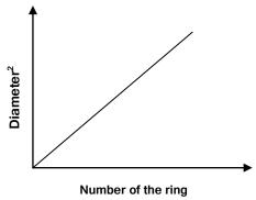
The value of  $\frac{D_m^2 - D_n^2}{4(m-n)R}$  is obtained from the graph. Radius of curvature of the Plano convex lens is measured with a spherometer. The values of  $\frac{D_m^2 - D_n^2}{4(m-n)R}$  and **R** are substituted in equation 1 to obtain the wavelength  $\lambda$  of monochromatic light.
