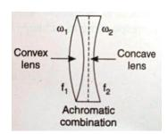
> To minimize chromatic aberration, ratio of focal lengths of the two lenses should be equal to the negative ratio of their dispersive powers.
