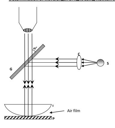
Consider a Plano-convex lens placed on a glass plate such that the convex surface of the lens touches the glass plate. Then an air film is formed between the convex lens and the glass plate. If a monochromatic light is incident on the air film normally, then alternate bright and dark concentric circular rings are produced due to interference. These rings are called Newton's rings.
